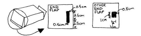
4. Cut 2 pieces of black electrical tape approximately 2" (5cm) long and stick it over the rectangular hole to form a narrow slit, 1mm wide.
